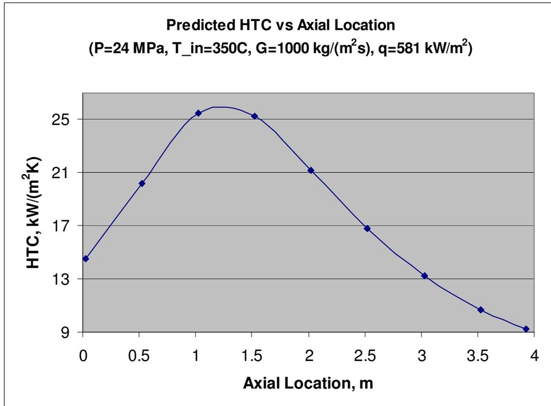
**Figure 3. Predicted dependence of heat transfer coefficient (HTC) on axial location along the heated tube length (Z-1) in the second modeling case.**
