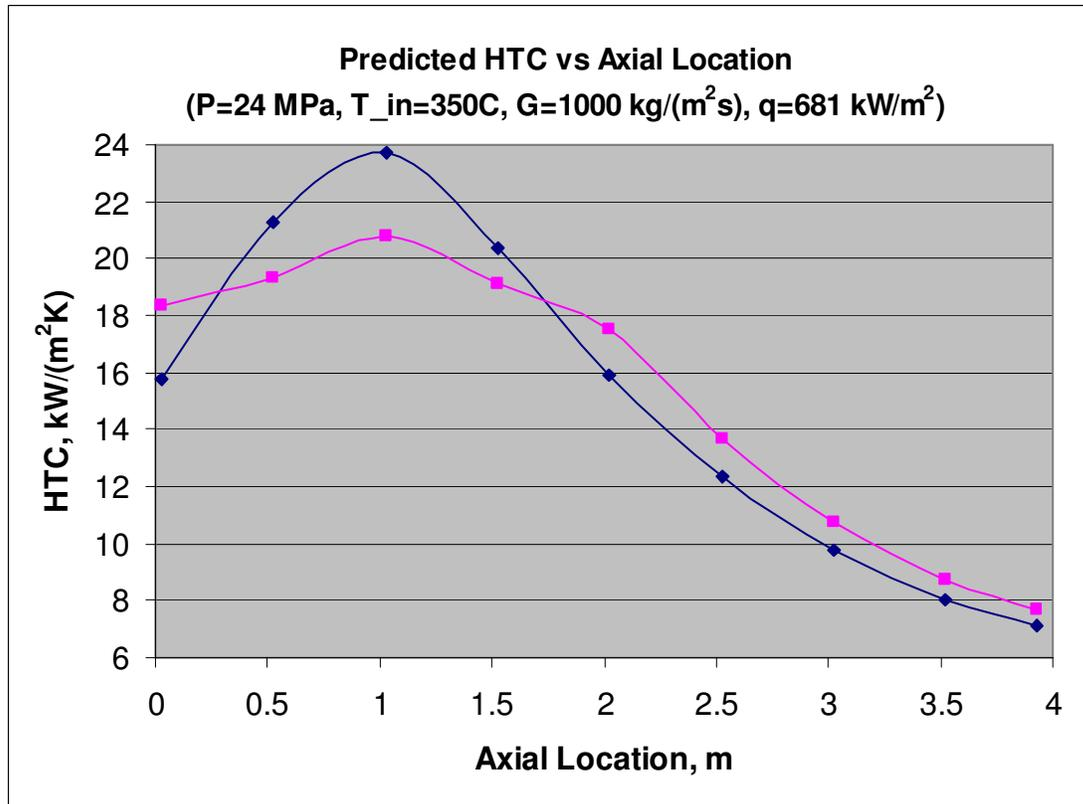
**Figure 2. Predicted dependence of heat transfer coefficient (HTC) on axial location along the heated tube length (Z-1) in the first modeling case (two different grids are used for comparison).**
