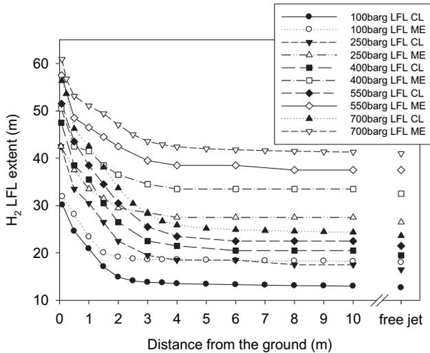
Fig. 4 – Lower flammability limit extent as a function of the leak proximity to the ground for hydrogen leaks (CL: Centerline extent; ME: Maximum Extent).
