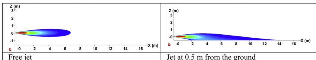
Fig. 3 – Contour of constant concentration (5% volume) of methane in air at steady state for the storage pressure of 100 barg.
