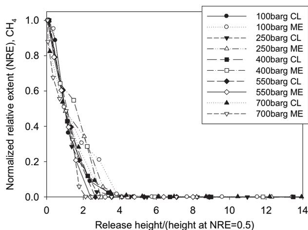
**Fig. 9 – Normalized Relative Extent (NRE) as a function of the release height normalized by the height at 50% NRE for methane jets (CL: Centerline extent; ME: Maximum Extent).**
