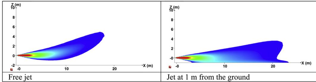
Fig. 2 – Contour of constant concentration (4% volume) of hydrogen in air at steady state for the storage pressure of 100 barg.
