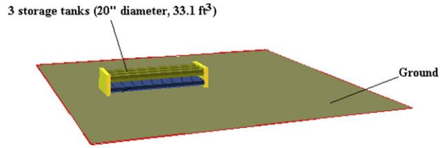
Fig. 6 – Storage geometry for hydrogen releases in PHOENICS at 100 barg.
