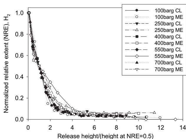
**Fig. 8 – Normalized Relative Extent (NRE) as a function of the release height normalized by the height at 50% NRE for hydrogen jets (CL: Centerline extent; ME: Maximum Extent).**
