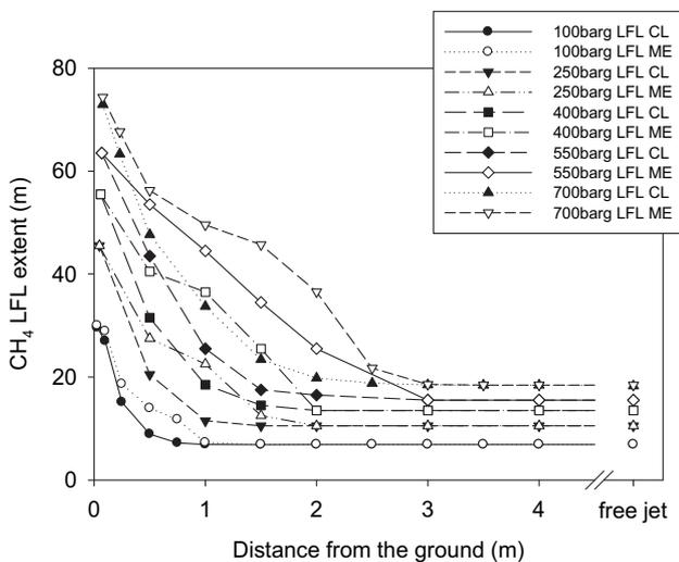
Fig. 5 – Lower flammability limit extent as a function of the leak proximity to the ground for methane leaks (CL: Centerline extent; ME: Maximum Extent).
