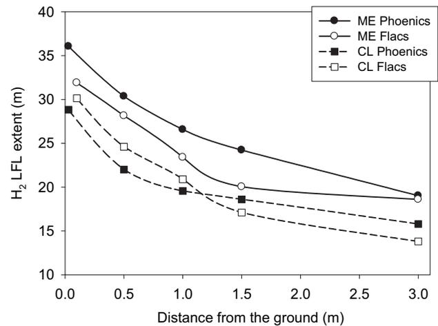
Fig. 7 – Comparison of PHOENICS and FLACS Hydrogen results for 100 barg leaks (CL: Centerline extent; ME: Maximum Extent).
