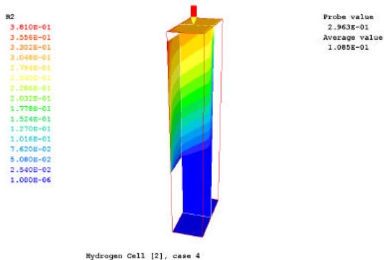
**Fig. 4. Gas volume fraction in Case 4:  $V_L=0.244 \text{ m/s}$ ,  $i=4.2 \text{ kA/m}^2$ .**
