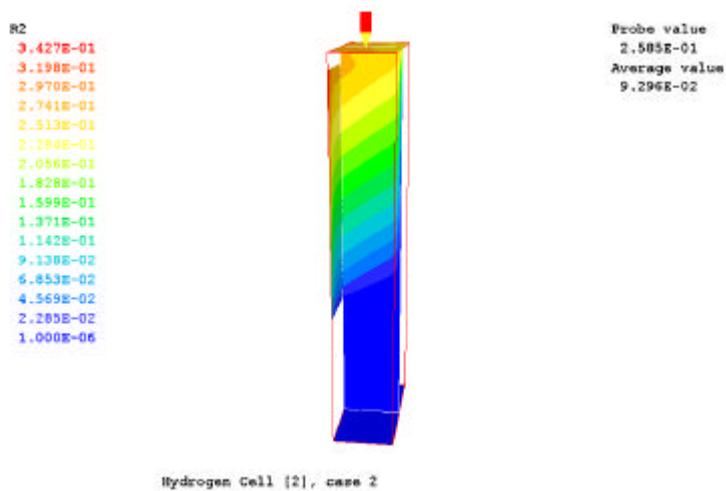
**Fig. 2. Gas volume fraction in Case 2:  $V_L=0.244$  m/s,  $i=3.5$  kA/m<sup>2</sup>.**
