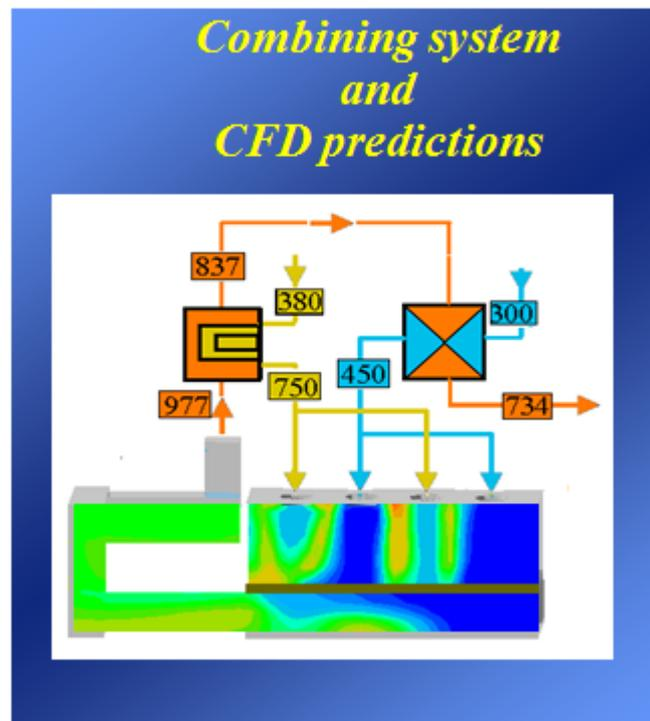
Most of the furnace operations are performed in thermo-technological loops/system where furnaces are surrounded with auxiliary and/or service devices such as heat exchangers [14]. As a rule the latter are fully coupled with each other and with, or through, a furnace. A screen snapshot shows one such system with two heat exchangers providing heat recovery.
