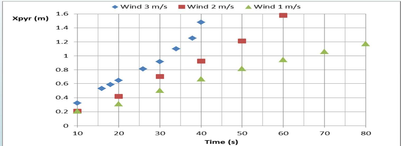
Figure 2. Pyrolysis front propagation for wind speeds of 1, 2 and 3 m/s
