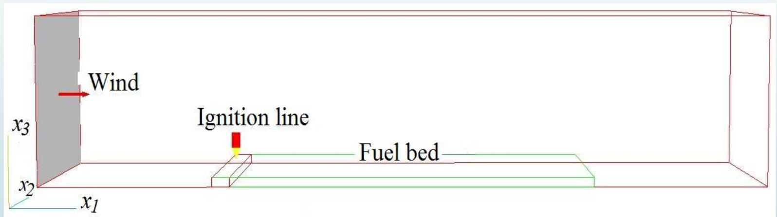
Figure 1. Computational Domain (wind, fuel bed and ignition line)
