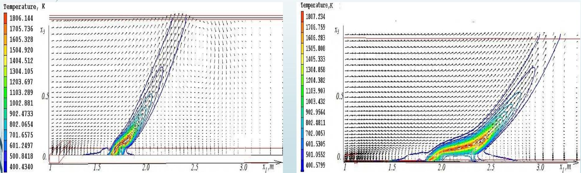
Figure 4. Gas temperature and velocity vectors at wind speeds of 1 m/s (left) and 2 m/s (right) at  $t = 40$  sec
