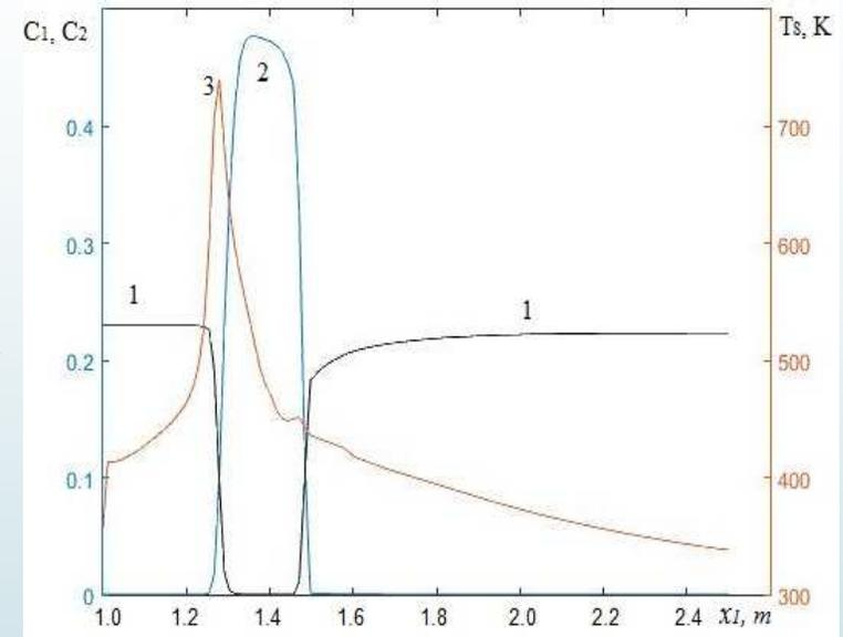
**Figure 3. Solid phase temperature (3) and mass fractions of oxygen (1) and carbon monoxide (2) for wind speed of 1 m/s**
