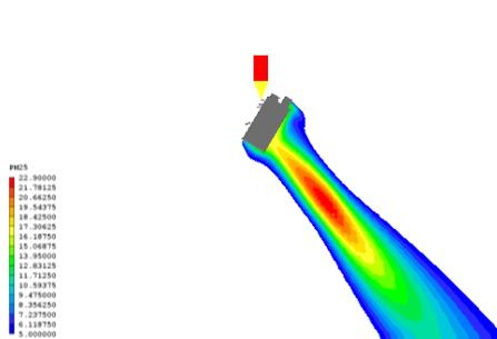
These results indicate that the increase in stack building heights decreased the maximum predicted concentrations of contaminants by about a factor of 4.2 based on the CFD model and a factor of 4.4 based on the CALPUFF model. Therefore, the effect of increasing stack and building heights on maximum predicted concentrations was similar for the two models.
