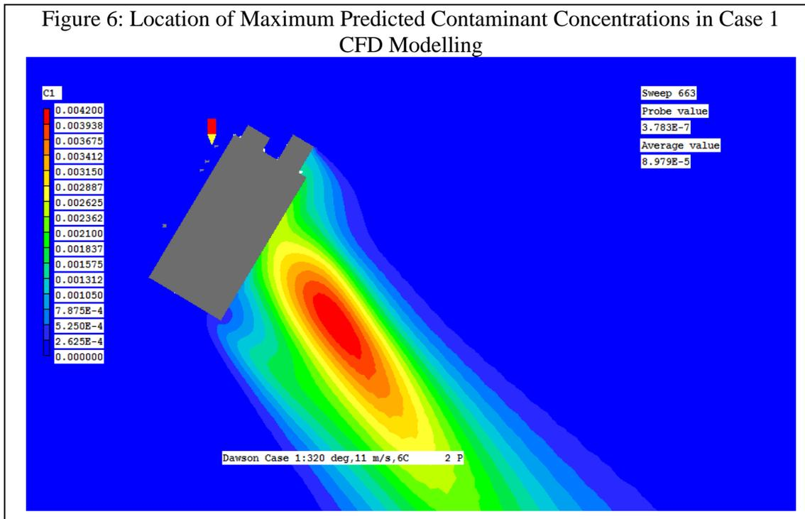
In order to verify the effect of lower wind speeds on maximum predicted NO<sub>x</sub> concentrations when four of the YEC engines are operating simultaneously, Case 1 was re-run three more times using the CFD model at varying wind speeds in order to determine the effect of wind speed on the maximum predicted NO<sub>x</sub> concentrations. These results are summarized in Table 9.
