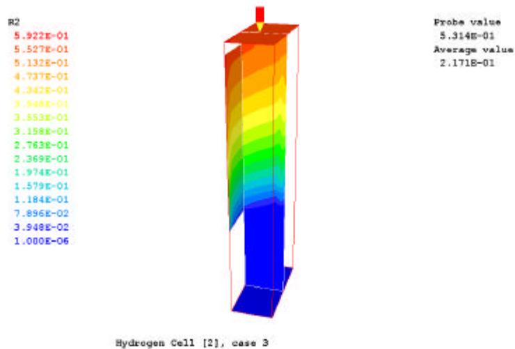
**Fig. 3. Gas volume fraction in Case 3:  $V_L=0.091 \text{ m/s}$ ,  $i=4.2 \text{ kA/m}^2$ .**
