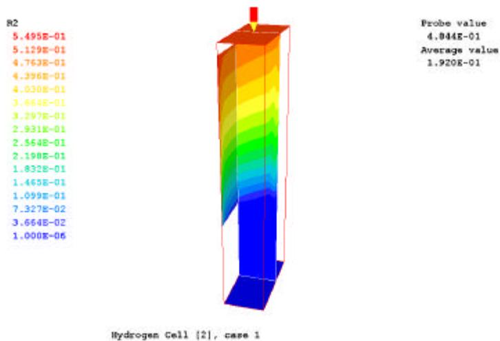
**Fig. 1. Gas volume fraction in Case 1:  $V_L=0.091$  m/s,  $i=3.5$  kA/m<sup>2</sup>.**
