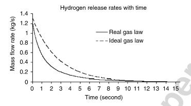
Fig. 3. Choked hydrogen release rate for the impingement release. Initial tank pressure: 700 bar. The leak orifice size:  $\frac{1}{4}''$ . Solid line: the choked release rate with using real gas properties (The predicted choked release lasts 14.14 s). Dash line: the choked release using ideal gas law (The predicted choked release release lasts 15.45 s). The ideal gas law overestimates the hydrogen release rate by up to 53% 3s after the onset of the release.
