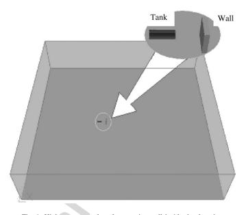
Fig. 1. High-pressure tank and preventive wall inside the domain.
