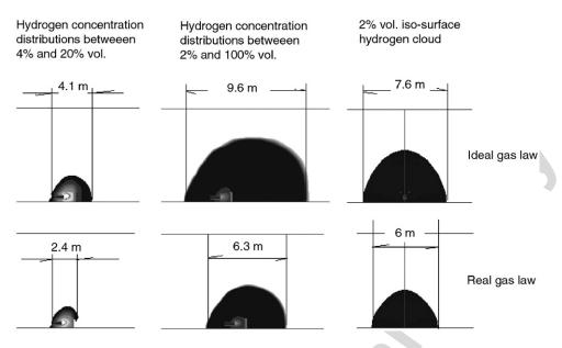
Fig. 6. Hydrogen cloud 5 s after the onset of release using ideal gas law and real gas law. Top three pictures: ideal gas law. Bottom three pictures: real gas law. Left: hydrogen concentration distributions between 4% and 20% vol on the plane that is in the direction of the release. Middle: hydrogen concentration distributions between 2% and 100% vol on the plane that is in the direction of the release. Right: 2% vol of hydrogen cloud iso-surface viewed in the direction of the release.
