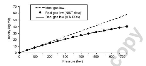
Fig. 2. Density deviation from ideal gas law as a function of pressure at 293.15 K. At 700 bar, the real gas density is about  $40 \text{ kg/m}^3$  but is overestimated by 45% when using the ideal gas law. Solid line: ideal gas law. Dots: NIST data [7]. Dash line: real gas law using AN-EOS.
