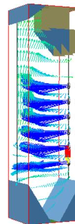
3d wall-fired 350MW lignite boiler
