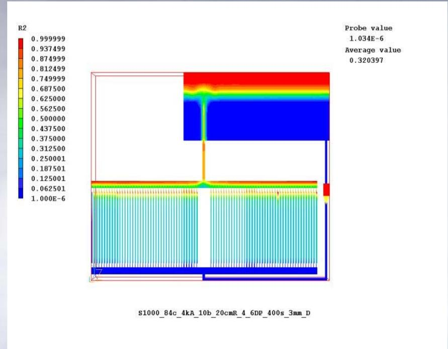
*Hydrogen volume fraction, R2, in commercial electrolysis system under standard operating conditions.*
